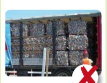
Not OK: void space not filled, not fixed, no lashing straps
